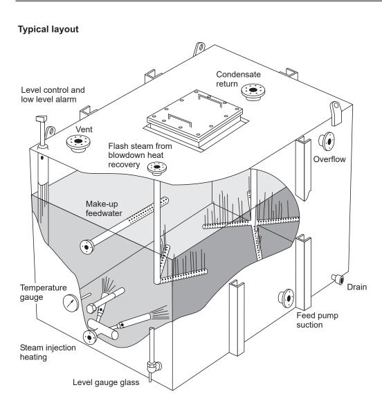
The Gestra Semi-Deaerator is a deaerating feedtank for heating and reducing the oxygen content of boiler feedwater
