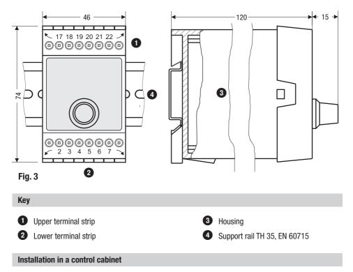
The TRS 5-52 temperature switch is clipped onto a TH 35, EN 60715 support rail in the control cabinet. Fig. 3 (
