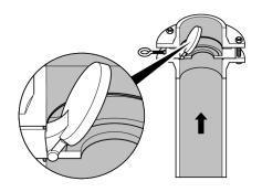
If the equipment is installed downstream of a pipe bend the eye bolt must point towards the inside of the pipe bend.
